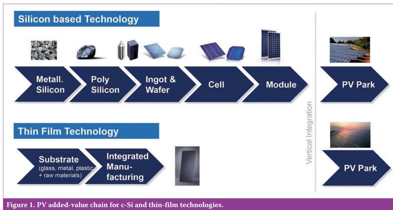
Figure 1. PV added-value chain for c-Si and thin-film technologies.
